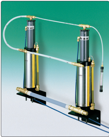
● Model 4675 High Sensitivity Settlement System.
